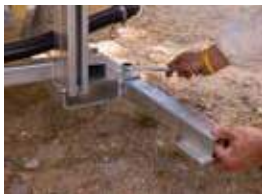
EASY ACCESS SLIDE-OUT PARKING LEGS FOR SAFE PARKING
